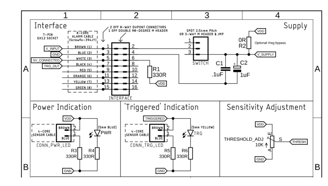
Timing Gate sensor board circuit (part 2)
