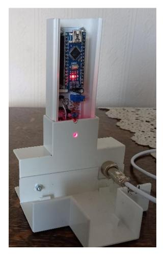
Rear showing yellow beam detected LED on
