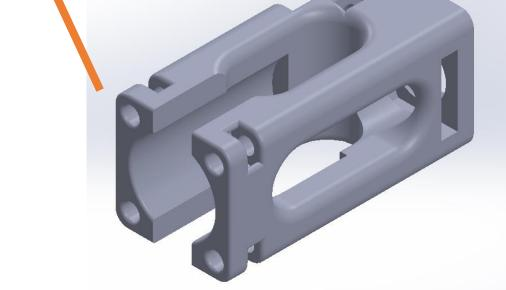
Optional 3D-printed support to give additional strength when removing plug from socket
