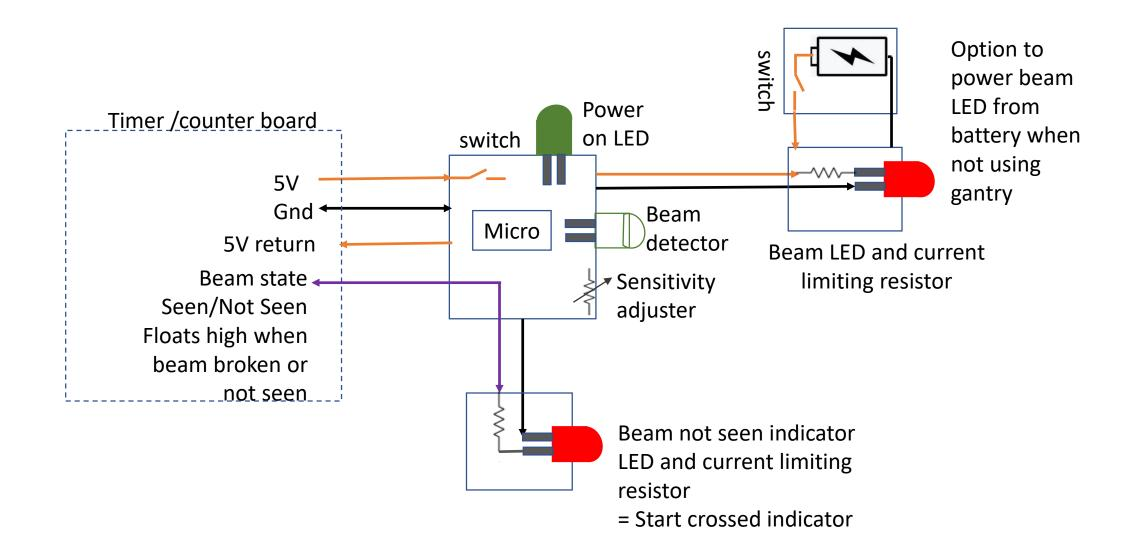
Reflector gate processor board components & interfaces For ½ size line follower course where not enough room for the beam LED on the course
